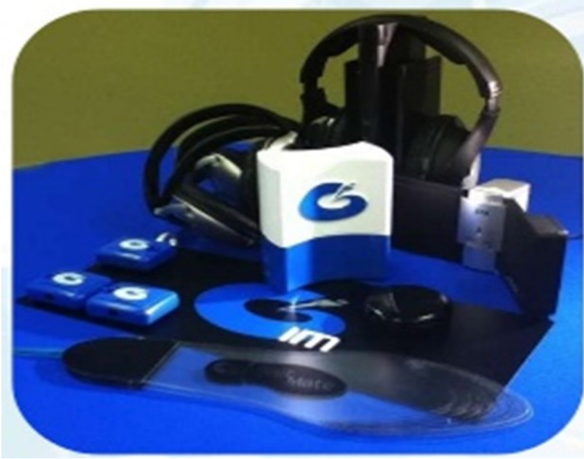
Fig. 1. The IM equipment consists of a software, a master control unit, a hand trigger, insole triggers, a tap mat, and headphones (Reproduced with permission from Interactive Metronome®)
